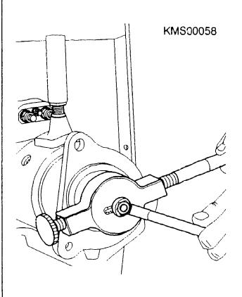
Disassembling control relay and starting-motor solenoid
